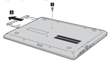
6 Remove the screw 3, then remove the optical drive bracket in the direction shown by arrow 4.
