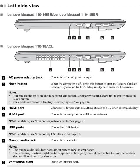
Note: Make sure that the ventilation slots are not blocked or else the computer may overheat.
