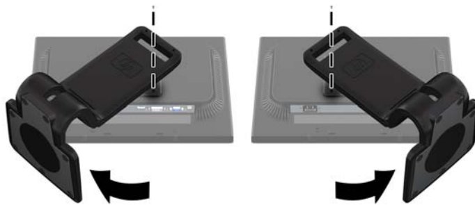
Figure 3-9 Removing the Pedestal Base Screws
