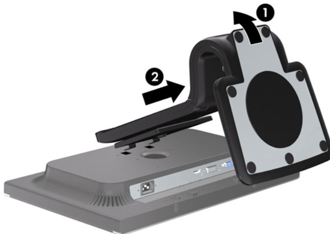
Figure 3-10 Removing the Pedestal Base
